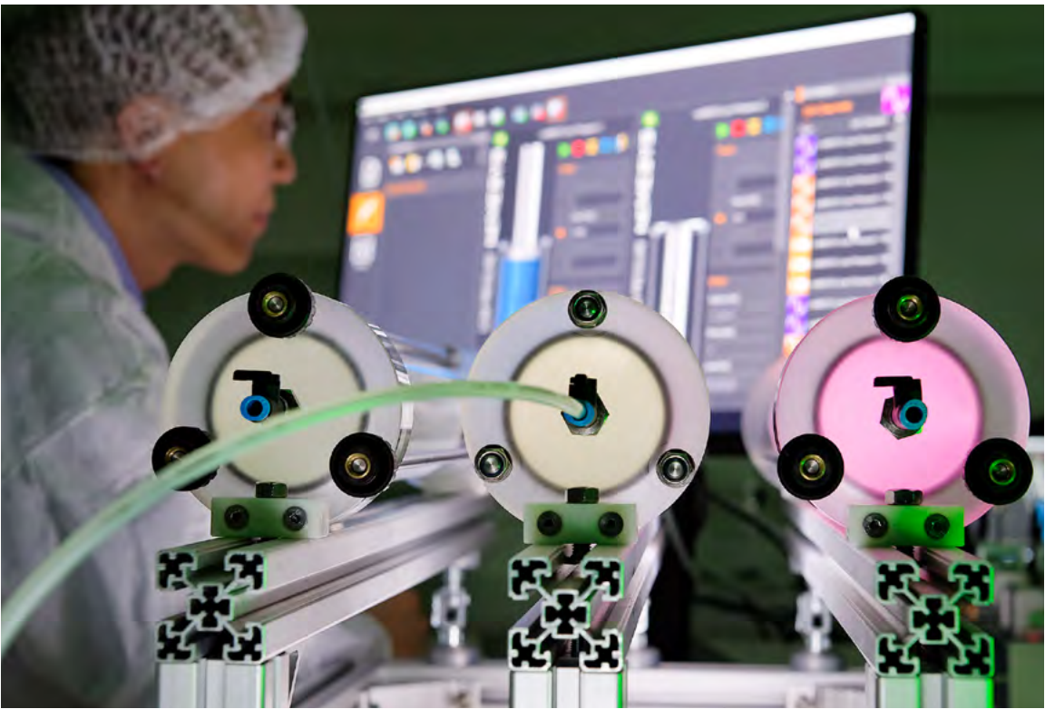
Testing the flow properties of various fluids (grey, yellow, pink) in a lab is quicker than testing in the actual rock layers.
